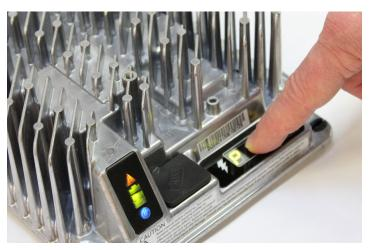
Press and release the Select Charge Profile Button to advance through the charge profiles. The selected charging profile will be displayed up to three times (e.g. "P-0-1-1" for Profile 11).\*
