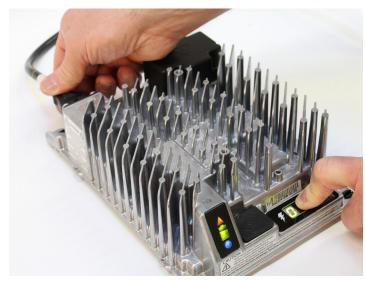
2. While reconnecting AC input, press and hold the Select Charge Profile Button. Hold the button (approximately 10 seconds) through the light check function until Error Indicator is on (in amber) and Battery Charging Indicator (in green) starts flashing.
